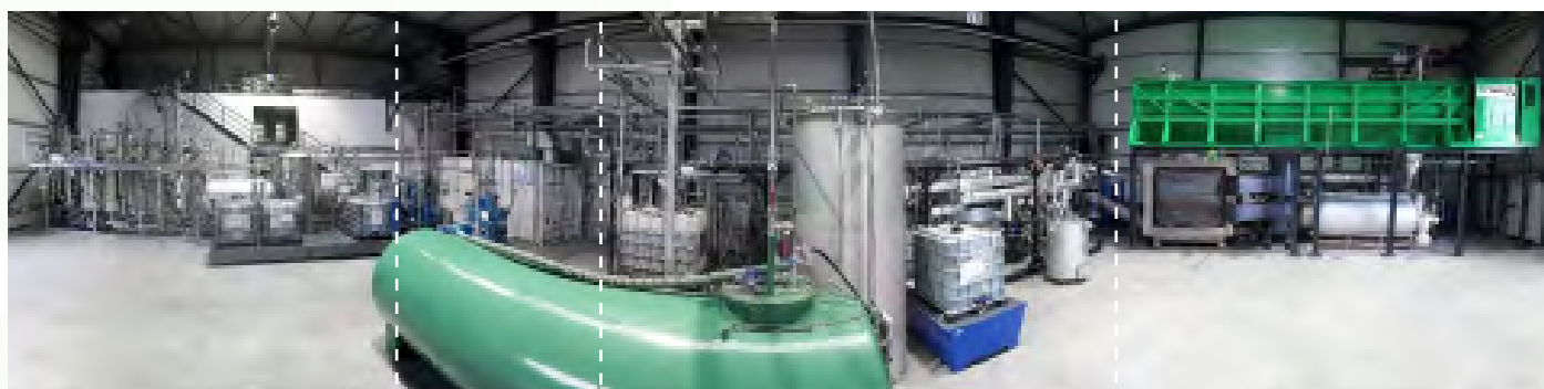
Complete process chain of To-Syn-Fuel-demonstrator: Hydrotreatment. PSA. Product gas train. TCR Auger reactor + Post reformer. Credits: Fraunhofer UMSICHT
